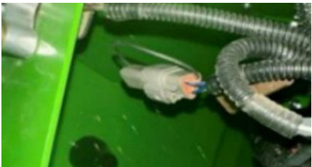
fig. 1C – CANDAapter shown connected to the CANbus port and USB on stand up models. VANQUISH's port is located under the tower below the display. FURY's port is located inside the controller compartment above the LH Drive Controller.
