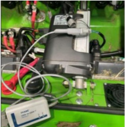
fig. 1A – CANDAapter shown connected to the RIVAL's CANbus port and USB near the RH Drive Controller under the seat.
