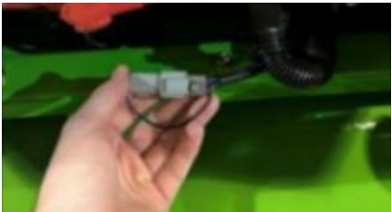
fig. 1B – CANDAapter shown connected to the EVO's CANbus port and USB located in the battery compartment near the RH Drive Controller.
