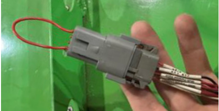
fig. 2B – 8 pin connector shown with jumper.
